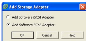
Figure 3.18 Adding a software FCoE adapter — Step 2 — vSphere 5.0 Client
