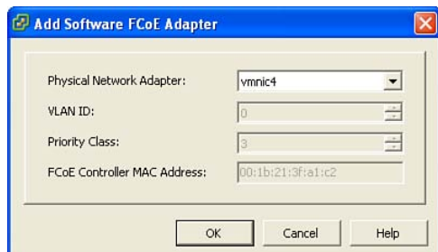
Figure 3.19 Adding a software FCoE adapter — Step 4 — vSphere 5.0 Client
