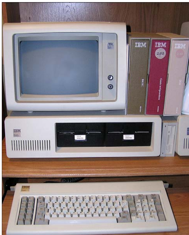
Figure 1.2 IBM PC (model 5150) shipped with two 5.25" floppy drives
