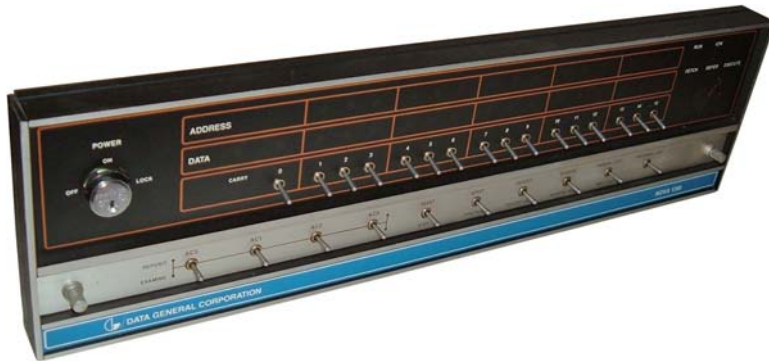
Figure 1.1 This photo of Data General’s Nova 1200 Mini Computer shows a 16-bit design (16 toggle switches).
