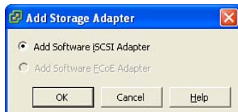
Figure 4.44 Adding an iSCSI SW Initiator—Step 2—vSphere 5.0 Client
